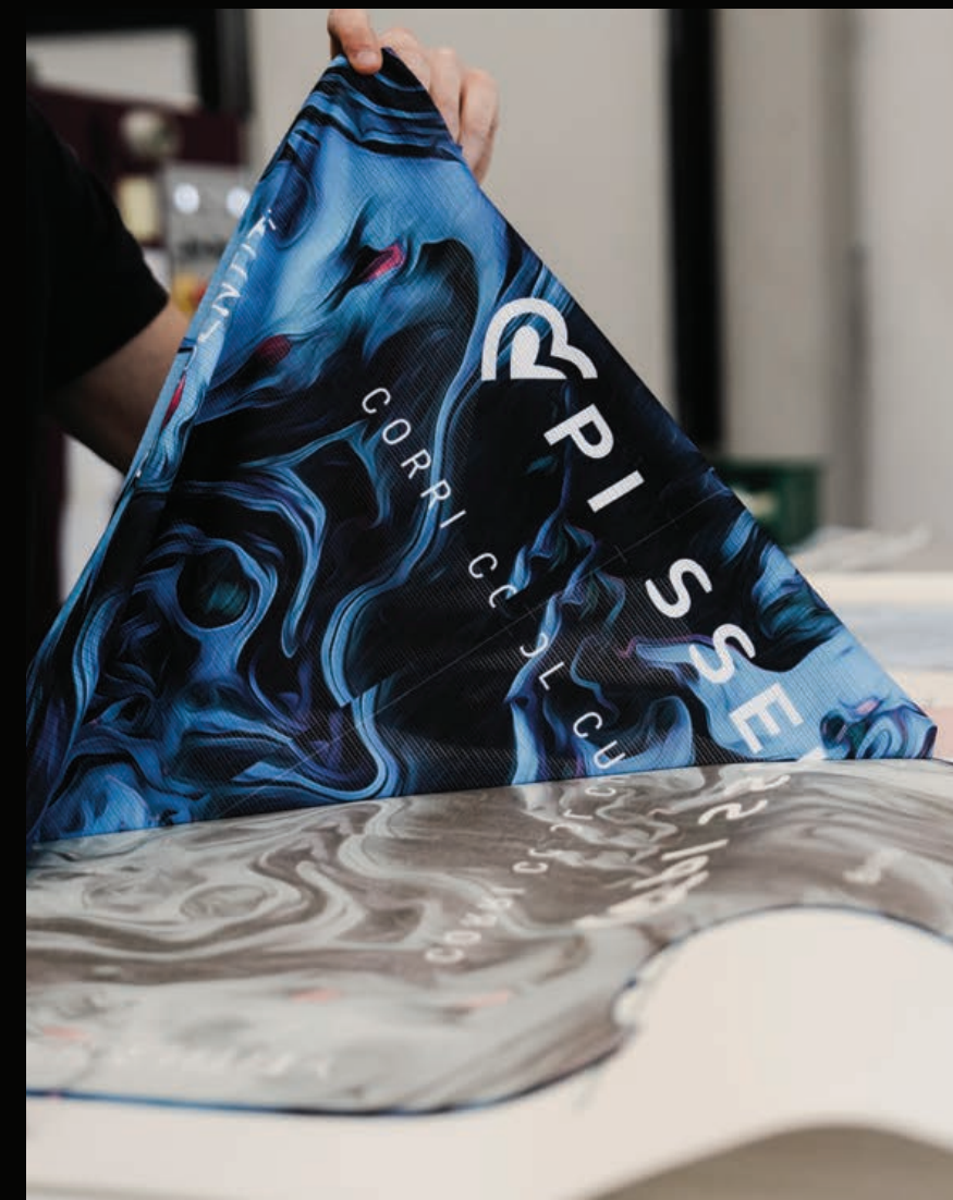
3.TRANSFER With a mixture of heat and pressure, the design gets transferred from paper the paper to
